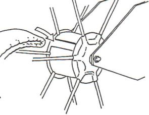
5 Wind hose over the top of the hub by turning reel as shown.
