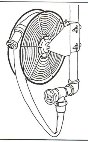
6 Connect female inlet coupling to hose valve.
