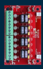
Provides 8 auxiliary power outputs, each one individually protected by a fuse (D8) or solid state circuit breaker (D8P).
