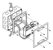
**GSA-MCC1S:** mount the UIOxR motherboard inside a suitable Kidde enclosure with screws and washers provided. Plug the module into any available position on the motherboard and secure the module to the motherboard with the captive screws. Wiring connections are made to the terminals on the motherboard (see wiring diagram). UIOxR motherboard terminals are suited for #12 to #18 AWG (2.5 mm<sup>2</sup> to 0.75 mm<sup>2</sup>) wire size.
