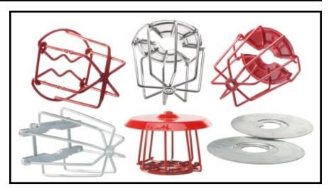
Model G1 and G4 Sprinkler Guards, G1/S1 and G4/S3 Sprinkler Guard with Shield assemblies, and S2, S4 and S5 Sprinkler Shields are compatible with specific types of Series TY-B, TY-FRB, TY-L, and TY-FRL sprinklers. See Table A. The Model G1 Sprinkler Guard in a stainless steel finish may also be used with the TYCO Type ULF Stainless Steel AM6 nozzle.
