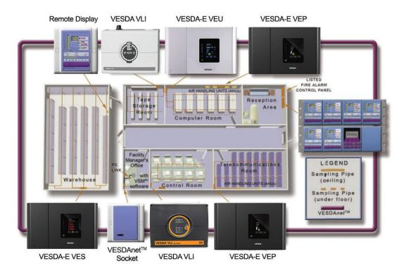
Having all VESDA smoke detectors on a VESDAnet loop allows you to configure and interrogate each detector from a central location, in this case the Facility Manager's office.
